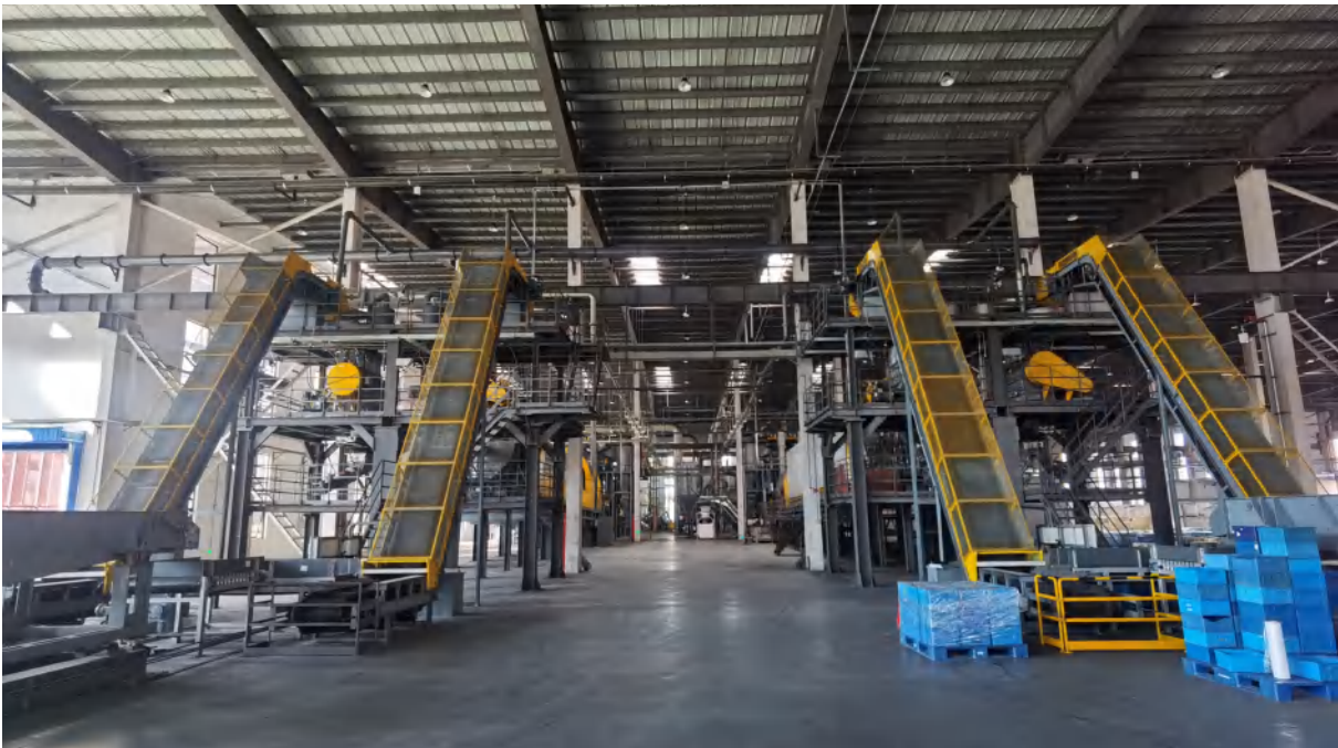
Waste Battery Cell Recycling and Crushing Line in Gotion Plant
